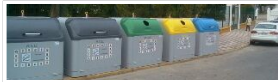
Metal containers with 3.000 litres of capacity for the selective waste collection: organic residues, glass, packaging and carton
