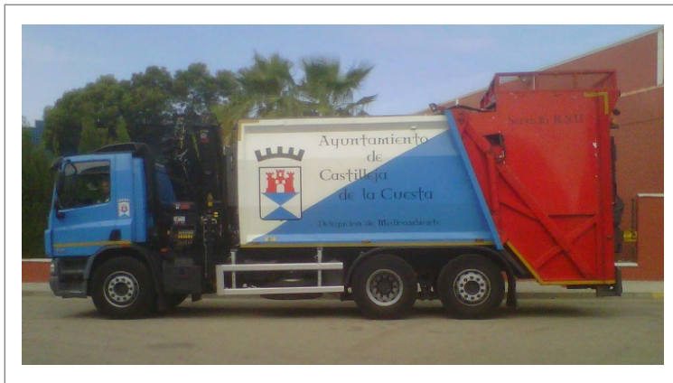
PV4 waste collector model with front crane on a 6x2 truck (brand Daf)
