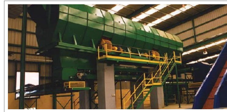
Lateral view of a waste classification trommel
