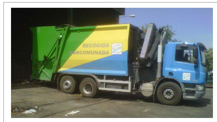
Another example of 6x2 truck with PV4 waste collector and front crane
