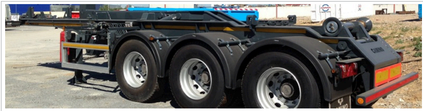
Trailer with multi-lifting equipment for the transport of high capacity compactors and waste containers
