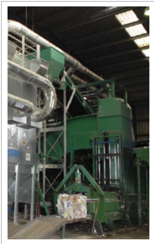
Pressing machine for making paper and carton bundles of optimal sizes
